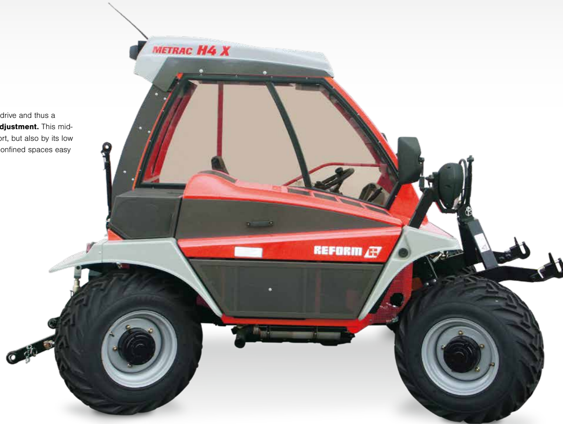
The Metrac H4 X has a front linkage with integrated lateral displacement as standard.
