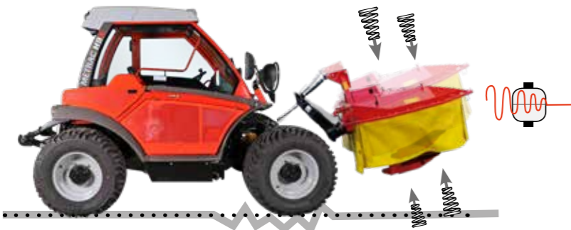
The impact load is minimised by gas pressure accumulators.
